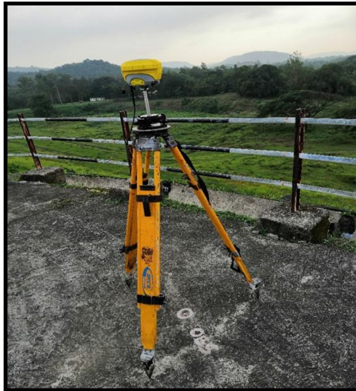
DGPS Observation At Dam Top
