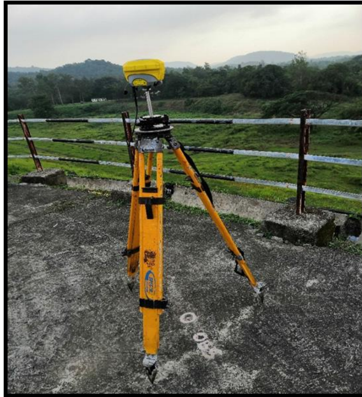
Figure 5.3-1 DGPS Observation at Dam top
